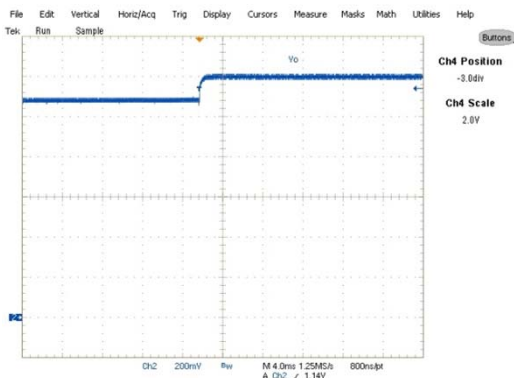
Fig. 9: Start up with 1V Pre Bias , 0A Load, Ch 2 : V_o
